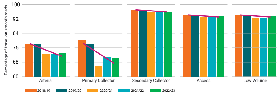
The percentage of travel on roads smoother than the threshold for each traffic grouping
