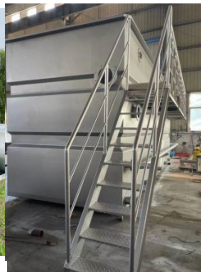
Figure 2: DAF unit being fabricated
