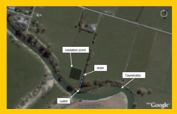
The Te Paerahi Wastewater treatment plant consists of an oxidation pond to treat the wastewater, prior to discharging through a wetland – discharging ontosand dunes.
