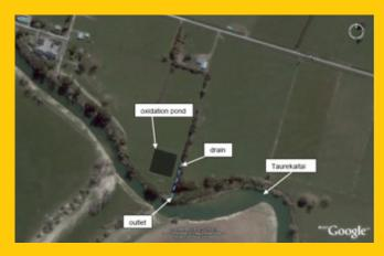
The Te Paerahi Wastewater treatment plant consists of an oxidation pond to treat the wastewater, prior to discharging through a wetland – discharging onto sand dunes.
