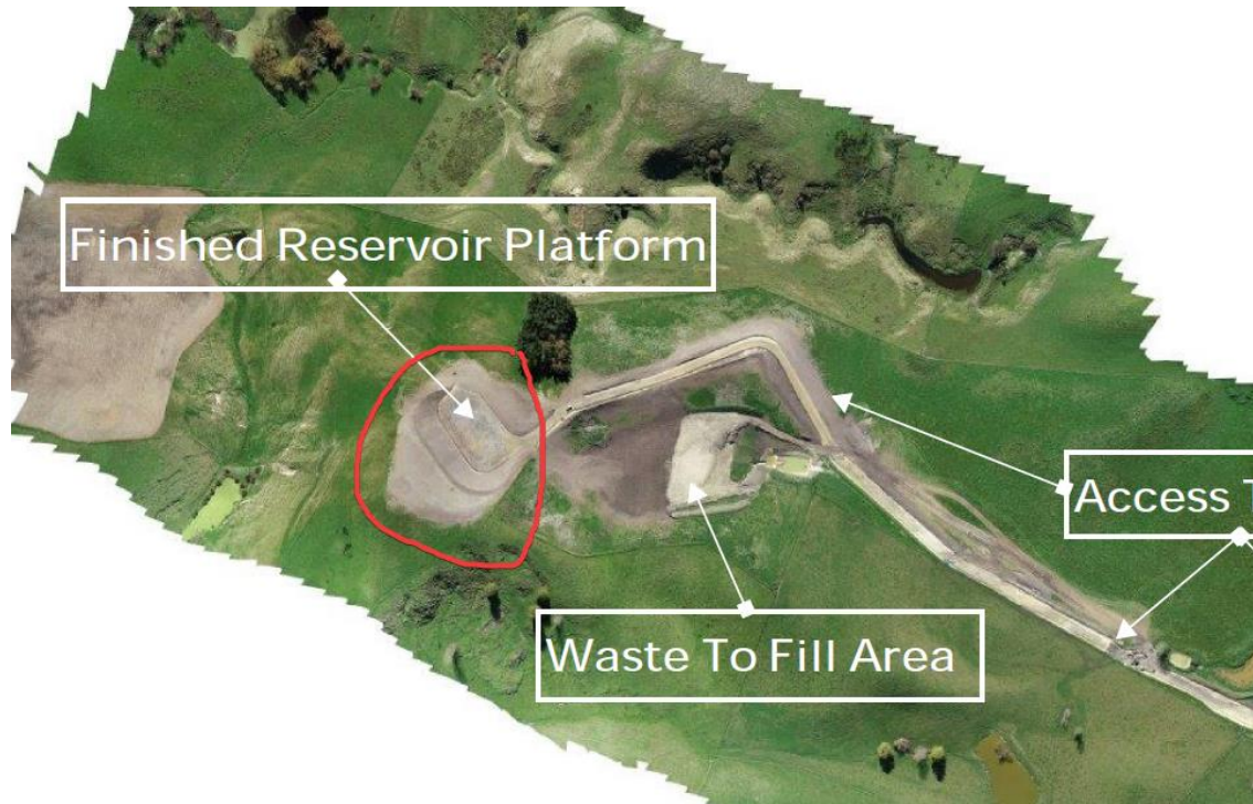
Figure 4: Site plan provided by Council (building platform shown in the red circle to correspond with map in Figure 3):
